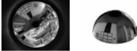
Figure 1. On the left a parabolic catadioptric image; on the right its 1:1 mapping to a hemi-sphere.
