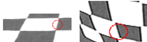
Figure 3. The images of a checker board part on a conventional image plane (left) and as obtained by a catadioptric system (right). Although it is not obvious the circular aperture of the right image contains a curvilinear edge.
