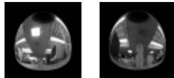
Figure 5: Rotated Images. Two spherical images from catadioptric images rotated relatively about the mirror’s optical axis.
