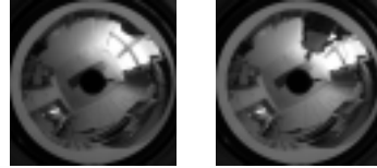
Figure 3: Clutter Images. On the left is a reference frame, and on the right is the same image with a human in the scene.
