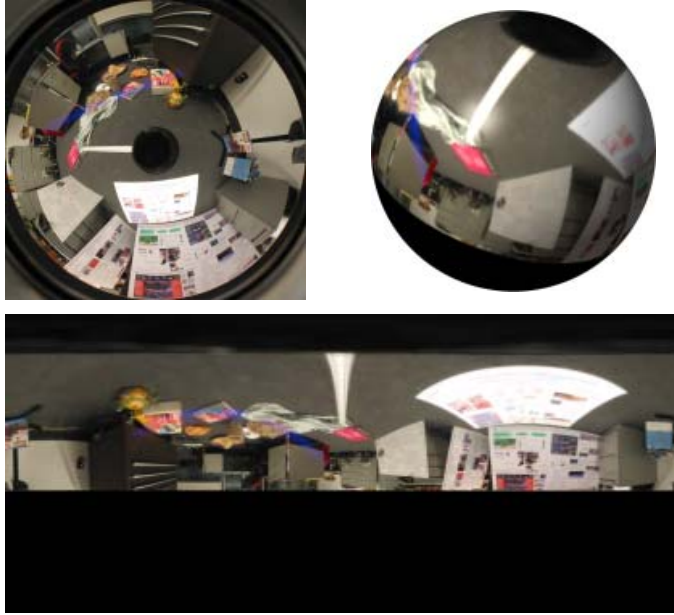
Figure 5: Top Left: a parabolic catadioptric image. Bottom: the corresponding image on a uniformly sampled spherical grid. As the parabolic mirror images only a little more than half the sphere, you can see the lower portion of the spherical image contains no information. Top Right: the spherical image as it would appear on the surface of the sphere.
