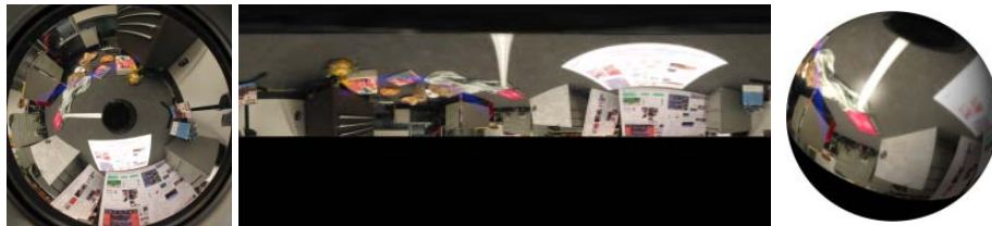
Figure 1: Left: a parabolic catadioptric image. Middle: the corresponding spherical image on a uniformly sampled spherical grid. Right: the spherical image as it would appear on the surface of the sphere
