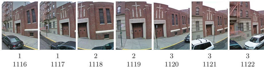
Fig. 1. A sequence of seven consecutive frames from our acquisition system that illustrates how the same scene content will be seen from multiple cameras over time separated by a wide baseline. At each of the seven time steps (frames 1116 through 1122), the same scene content is observed from one of the three cameras (1, 2, or 3). With frame-to-frame feature matching we are more likely to generate tracks that observe world points from very different viewpoints angles than if we tried to match features directly between the extreme wide baseline image pairs.
